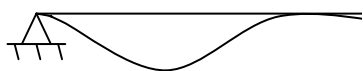
Figure C.2. Moment distribution in the early stage of a beam subjected to an impulse load. Due to the rigid body response the moment is zero in the midpoint.
