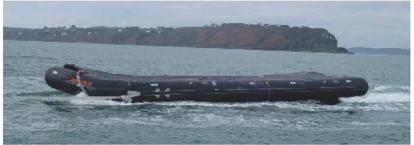
Floating oil storage barge 100m 3
